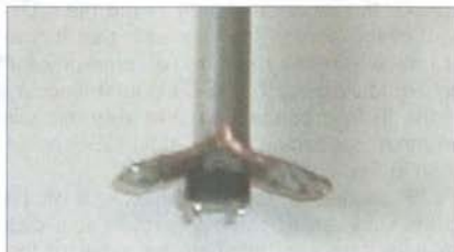
Fig. 3: Diode soldered to inner connector
