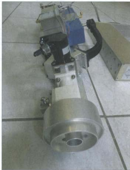
DL7YC Horn with 10G Transverter-block
