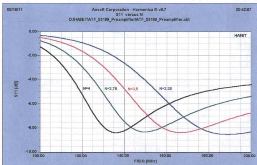
Fig. 6: S11 versus number of inductor turns, N (simulation)
