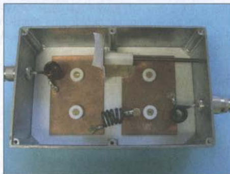
Fig. 5: Low Pass Filter by F1TE
