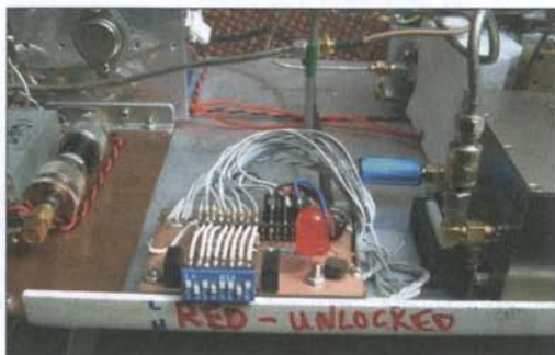
Fig. 9: DIP switch for the YIG Oscillator
