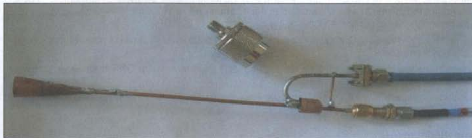
Fig. 1: Homebrew 3 port coaxial harmonic mixer
