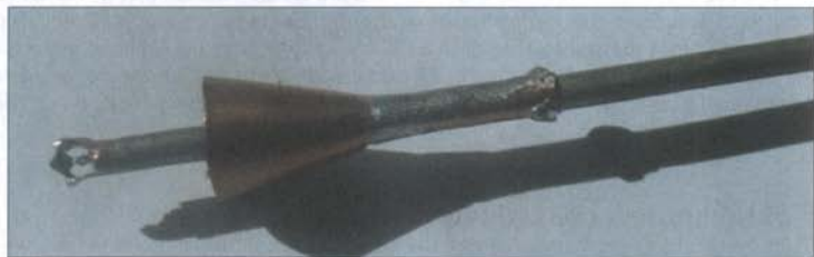
Fig. 5: Feed horn with sliding collar on the hardline
